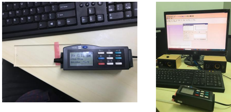
Figure 4. Thermoplastic Nylon Surface Roughness Testing in the Laboratory
