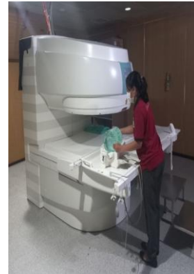
Image 1. Placement of the phantom on the MRI Head Coil
