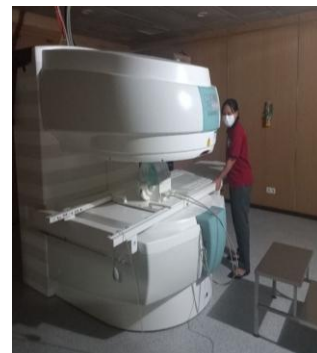
Image 2. Placement of the phantom at the center of the MRI magnet bore
