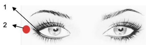
Figure 7 Third Area for Radiation Dose Measurement Around the Eyes of the Head Phantom
