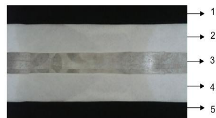
Figure 3 Layers of Eye Radiation Protection Devices
