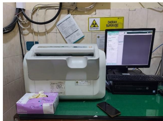
Figure 3. Computed Radiography Devices (Computer and Reader) in the Radiology Installation of Kendal District Hospital
